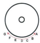
Orientation A to G at equidistance of 200 mm with location D at bottom
